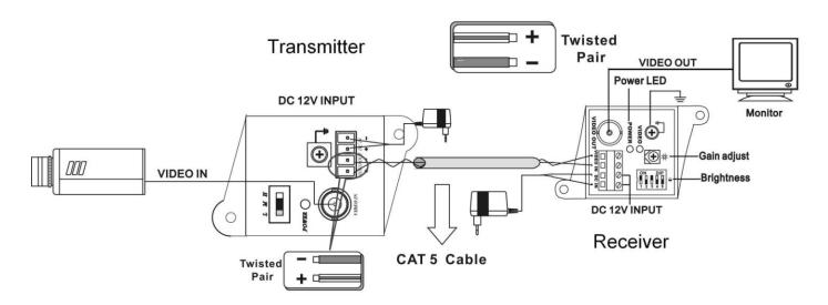
\*The unit built in transient protection, please make sure to make grounding.
